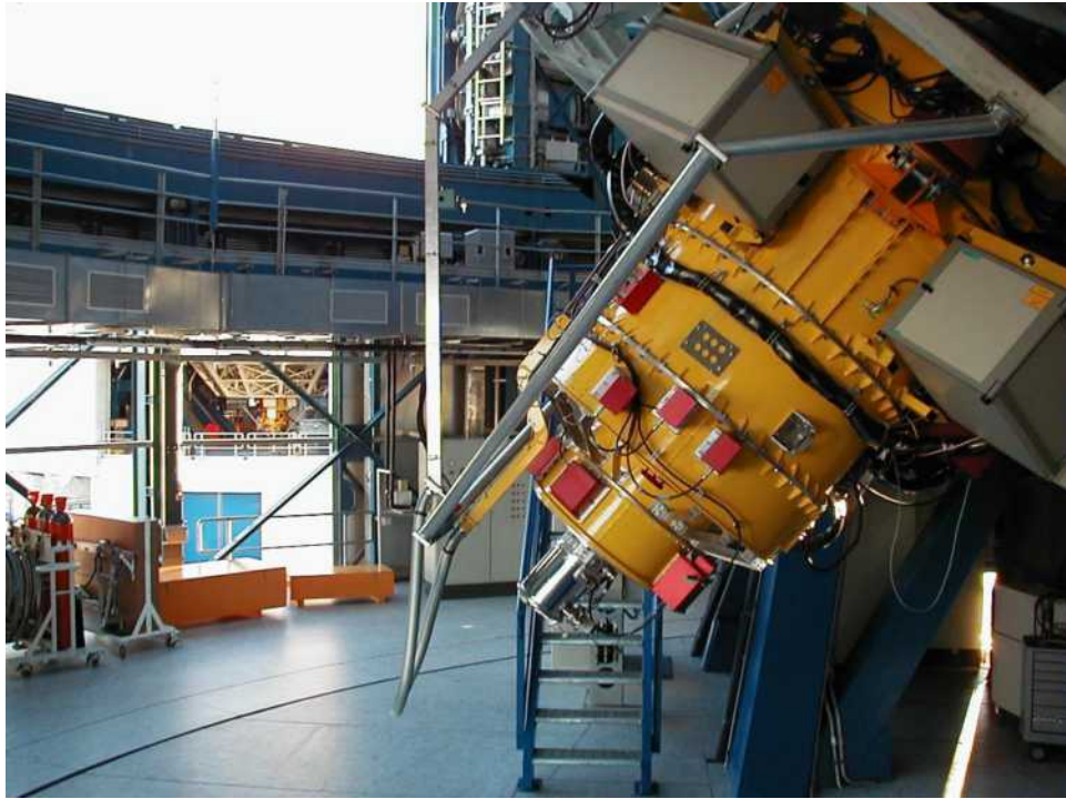
Figure 2.1: The twin FORS instruments. FORS2 is shown in the foreground at the Cassegrain focus of UT2 , and the now decommissioned FORS1 instrument is visible in the background, at the same focus of UT1 . In 2009 FORS1 was decommissioned to make room for the first of the second generation instruments at the VLT , namely X-shooter , where FORS2 was then moved to its current location. © ESO
